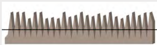
Fig.11-Pic.11: R_a = 0,4 \mu\text{m}/16 \mu\text{m} R_{MR} : 15%
