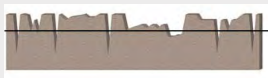
Fig.12-Pic.12: R_a = 0,4 \mu\text{m}/16 \mu\text{m} R_{MR} : 75%
